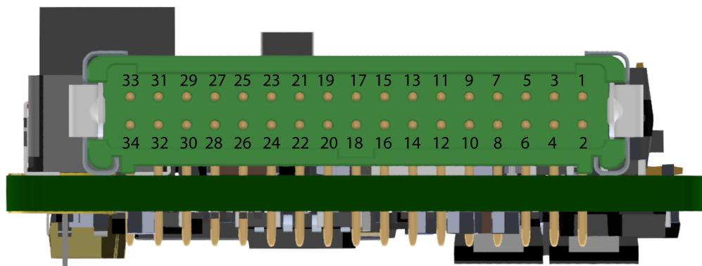
**MEX connector pinout**
