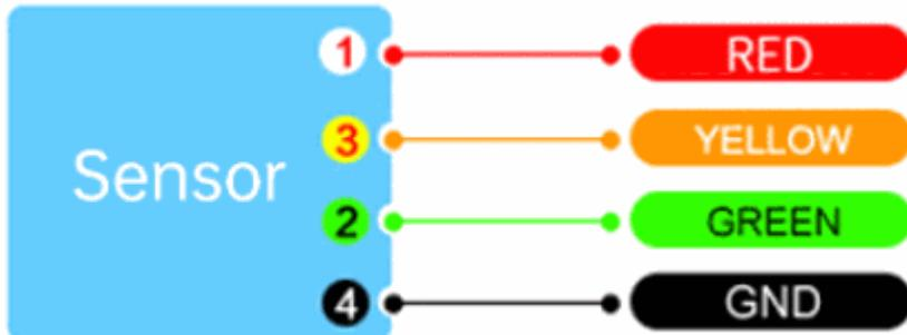
WitMotion HWT905-232 connector pinout
