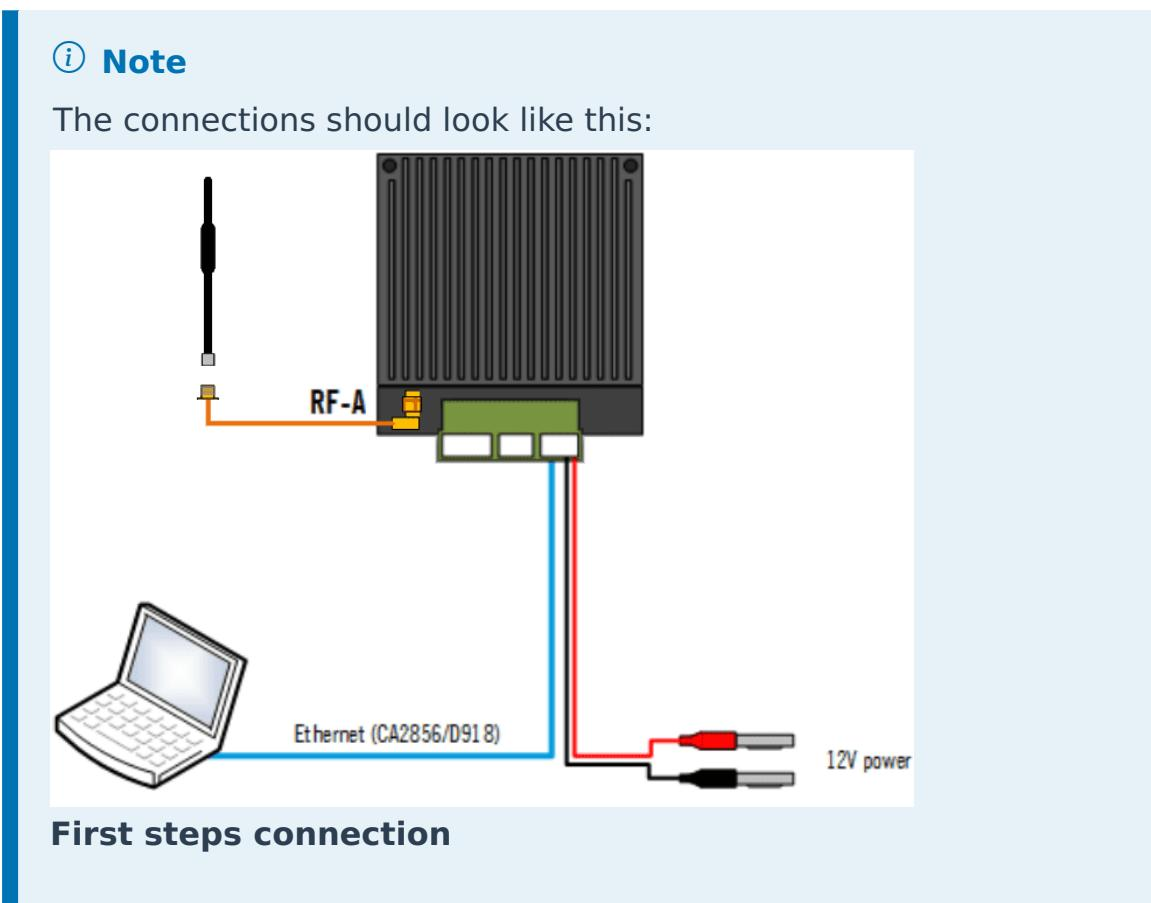
1. Make sure computer is set to static IP address on same subnet as radio. The following substeps clarify how to set the IP address in the **Control Panel**:
