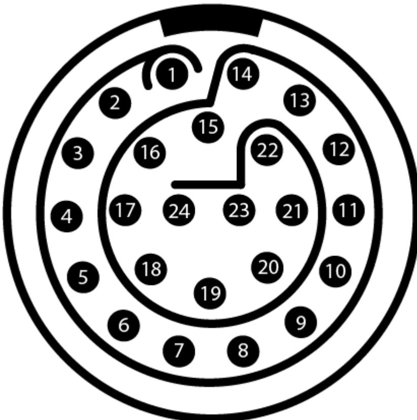
**MC24 connector pinout**
