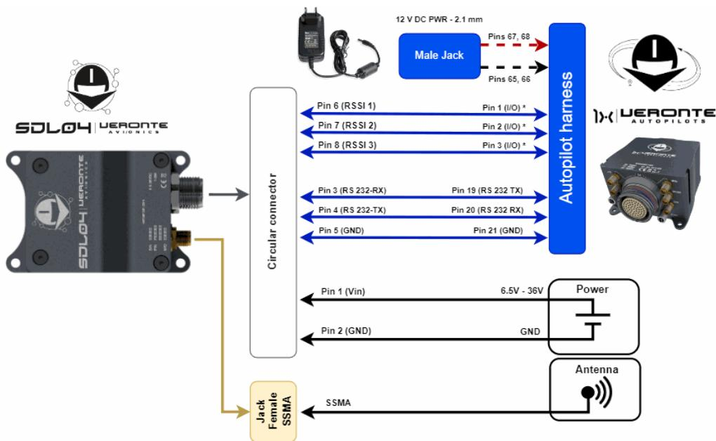
\* Those signals are configurable I/Os, so they can be connected to the following 1x pins instead: 1, 2, 3, 4, 5, 6, 7, 8, 10, 11, 12, 13, 14, 15, 16 or 17 (NOT 9)
