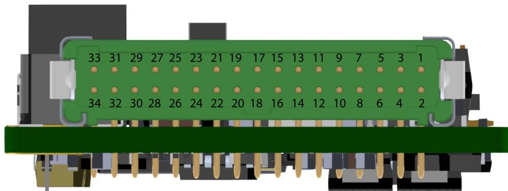
MEX connector pinout
