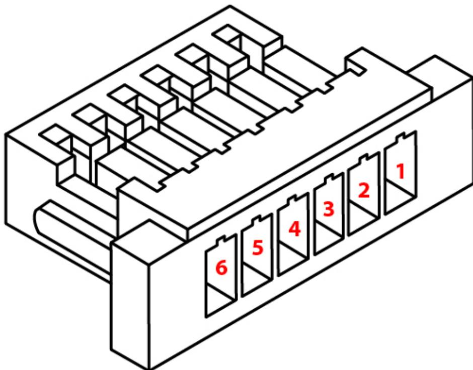
**J3 (RS232) pinout of female connector**
